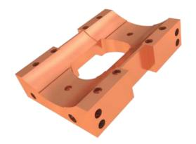
The "Forged" Type is produced by making a specific forge mould or directly by forging a copper block or a semi-prepared moulded part which its dimensions are close to the final one; this model's electrical conductivity is above 101% of IACS and is more consistent. Thus, the forged model is more reliable compared with the Moulded one and of course, final price is higher compared with moulded types.
